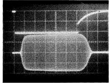
Fig. 3 — The keyed cw waveform of the Kenwood TS-180S. The horizontal divisions are each 5 ms. The upper waveform displays the actual key-down time. Such a smooth waveform should not have any clicks.
