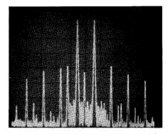
Fig. 2 — Output display of the '180S during a full-power 14-MHz two-tone test. Each vertical division is 10 dB and each horizontal division is 1 kHz. The third-order distortion products are down 38 dB from the PEP level.
